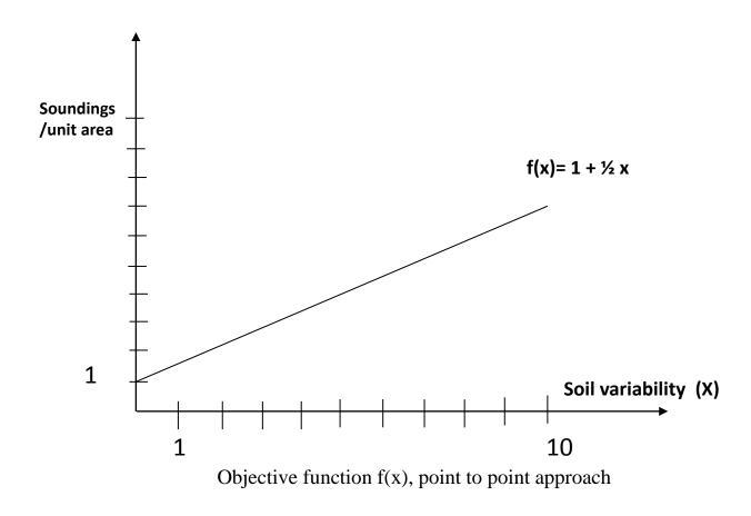
The obtained "objective function" permits to calculate the number of soundings based on soil variability
