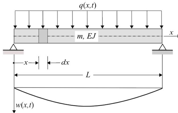
Figure 1. Geometry of the uniform beam with symmetrical load.
