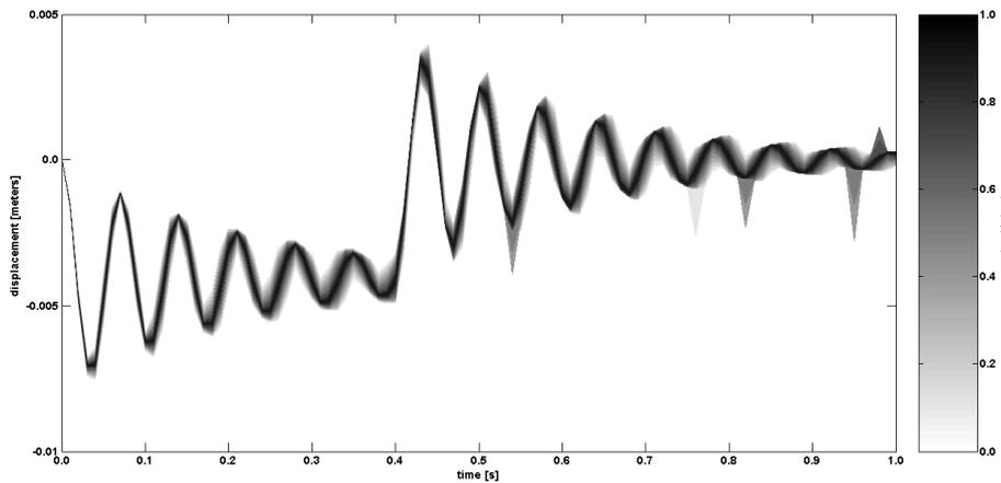
Figure 6. Vertical displacement of the midspan with  $\mathbf{p}_1 = \mathbf{p}_2 = [0.95, 1.05]$ ,  $\mathbf{p}_3 = [1.0, 1.0]$  and 5 percent damping.
