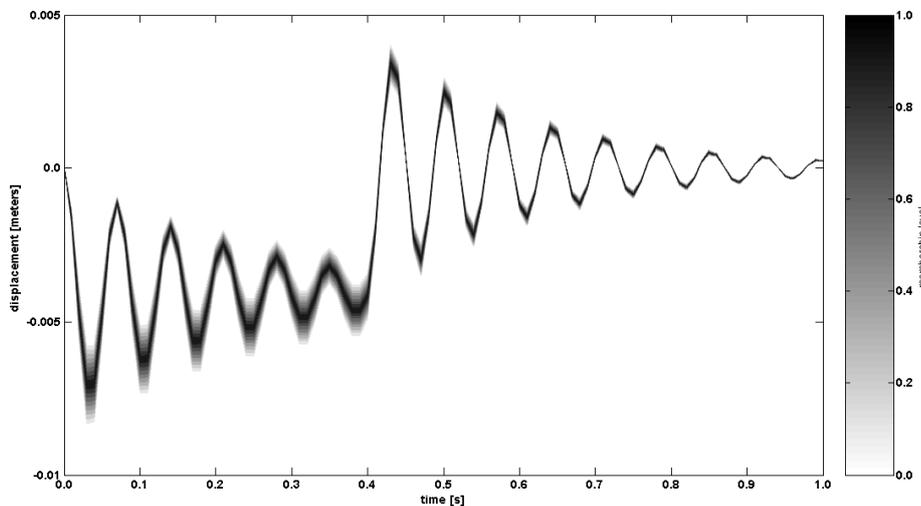
Figure 7. Vertical displacement of midspan with  $\mathbf{p}_1 = \mathbf{p}_2 = [1.0, 1.0]$ ,  $\mathbf{p}_3 = [0.8, 1.2]$  and 5 percent damping
