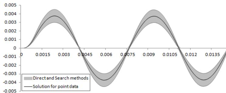
Figure 5. Vertical displacement of the midspan; comparison of the results of Direct method and Search method for the case:  $E = 200[\text{GPa}]$ ,  $\rho = 7850[\text{kg/m}^2] \pm 0.5\%$ ,  $q \approx 2.5[\text{kN}] \pm 20\%$ ,  $n_x = 20, n_t = 100, \Delta t = 0.0015$ .
