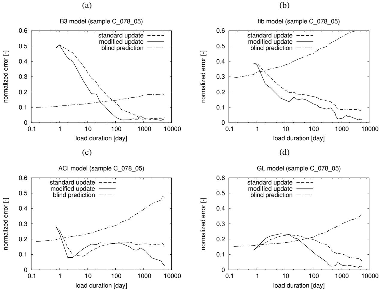
Figure 2. Normalized residual error  $e_u^{(m)}/J(t_0 + 1000, t_0)$  as a function of the load duration up to the updating time,  $t_m - t_0$ , for Water Tower Place concrete: comparison of the blind prediction with the standard and modified updates for (a) B3 model, (b) *fib* model, (c) ACI model, (d) GL model.
