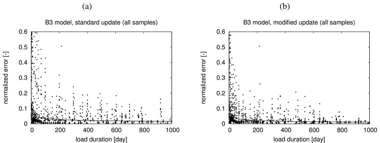
Figure 4. Normalized residual error of updated B3 model for all tests considered: (a) standard updating, (b) modified updating.
