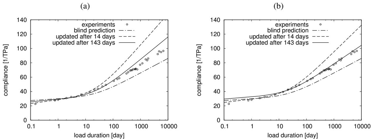
Figure 1. Compliance function of Water Tower Place concrete: (a) standard updating with equal weights of all measured points, (b) modified updating with the weight of each measured point proportional to the duration of loading.
