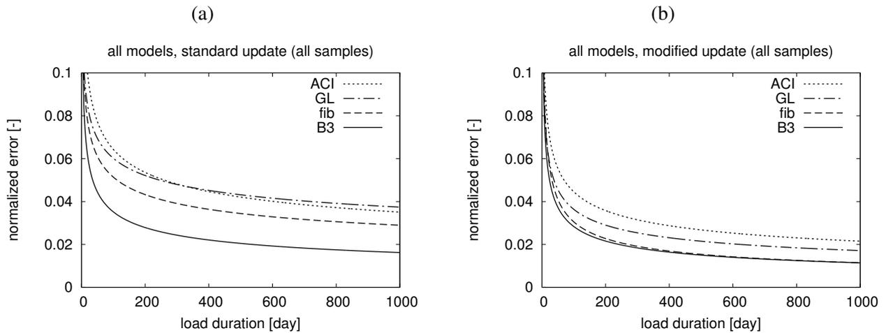
Figure 5. Comparison of power-law curves approximating the average normalized residual error for different models: (a) standard updating, (b) modified updating.
