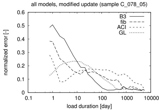
Figure 3. Normalized residual error  $e_u^{(m)}/J(t_0 + 1000, t_0)$  as a function of the load duration up to the updating time,  $t_m - t_0$ , for Water Tower Place concrete: comparison of modified updates for individual models
