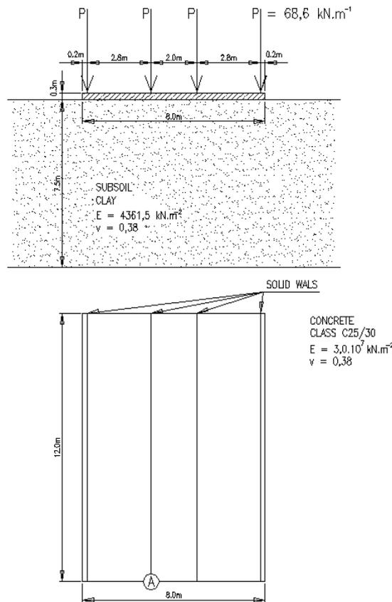
Figure 1. Foundation slab with longitudinal walls
