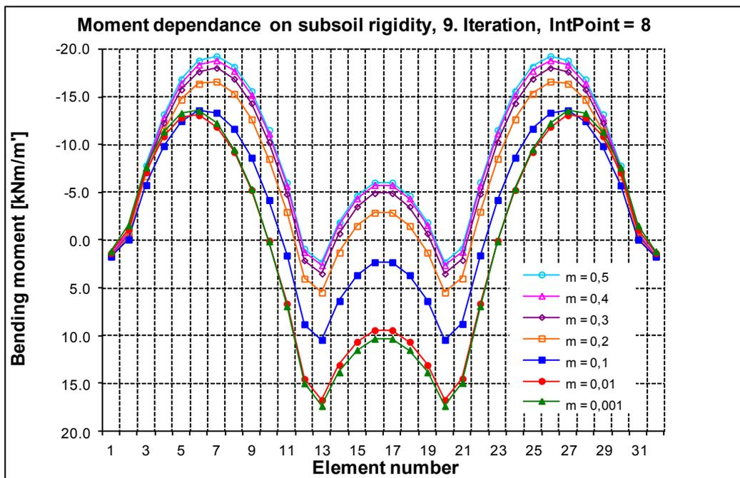
Figure 6. Transversal moment vs. structural strength of the soil in subsoil and depth of the deformation zone if a contact element is used
