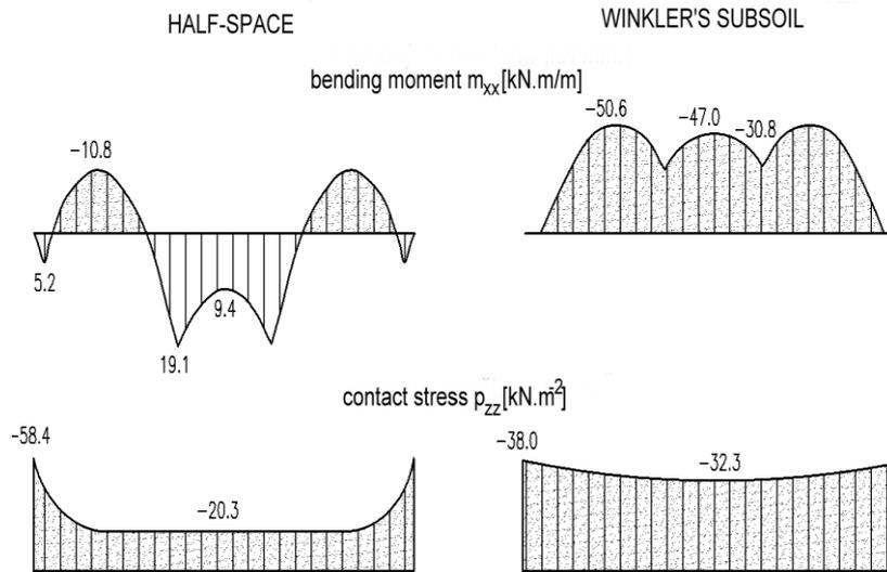
Figure 2. Internal forces in the transversal direction obtained by solution of a slab in a subsoil model with 3D elements and in a Winkler's subsoil model according to 1
