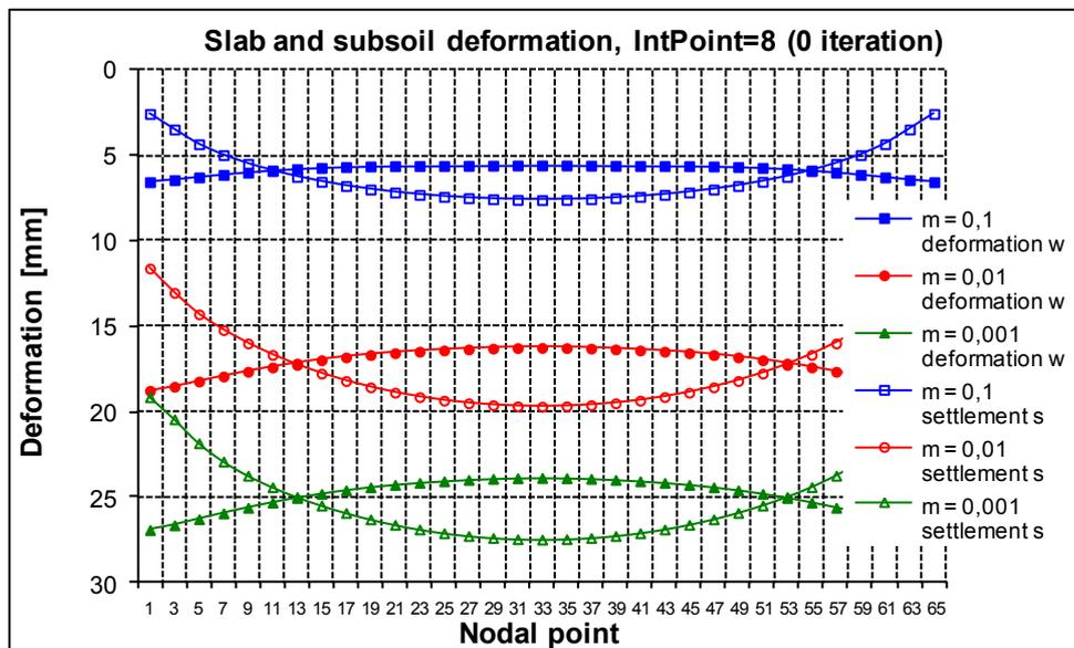
Figure 3. Deformation of the slab and settlement of subsoil vs. structural strength of the soil in subsoil of a contact element – without iterations
