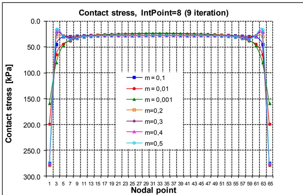
Figure 5. Contact stress vs. structural strength of the soil in subsoil and depth of the deformation zone if a contact element is used – 9<sup>th</sup> iteration
