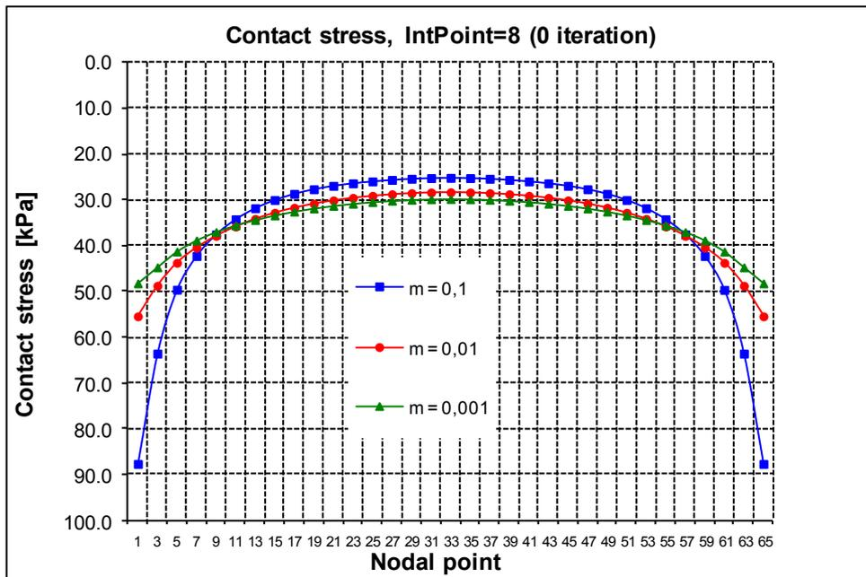
Figure 4. Contact stress vs. structural strength of the soil in subsoil and depth of the deformation zone if a contact element is used – without iterations
